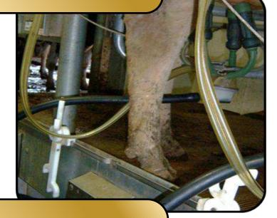
Parabone stall angle is made by simply twisting the top branch of the tree. The Parabone Slender Hose Tree can also be used to milk from the side of the cow.
